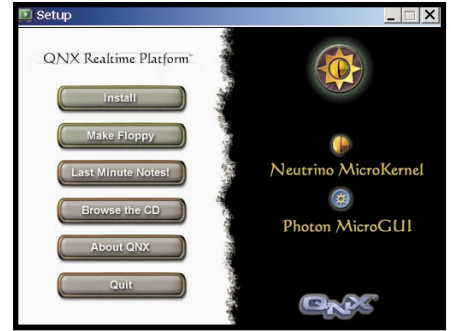
Photo 2 —You can install QNX Neutrino from Windows to a Windows FAT partition. The installation window also gives an option to make boot floppy disks, should you want to install the system on a QNX partition and your system does not support booting from a CD-ROM.
